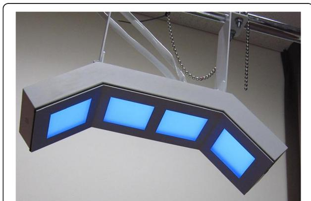
**Fig. 1** Lighting device with organic light-emitting diode (OLED). The device consists of four OLED panels (55  $\times$  55 mm<sup>2</sup>) with adjustable red-green-blue color and brightness. The panels are linearly aligned and two panels at the both sides incline inward with an angle of 40°
