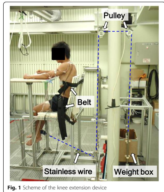
**Fig. 1** Scheme of the knee extension device
