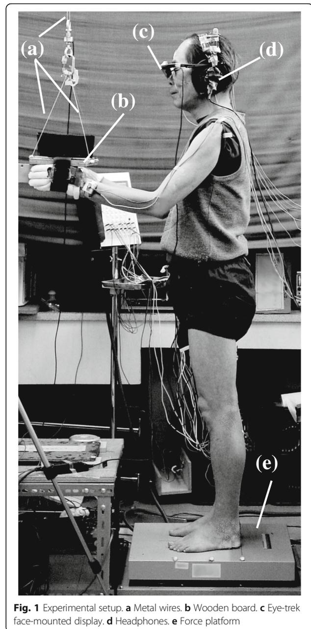
**Fig. 1** Experimental setup. **a** Metal wires. **b** Wooden board. **c** Eye-trek face-mounted display. **d** Headphones. **e** Force platform
